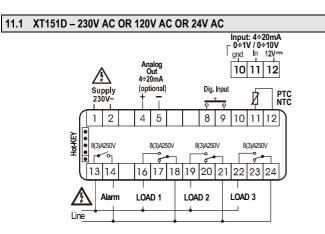
Probe: Pt100=11 - 10 (12); Thermocouple J, K, S= 11(+) - 10(-) 115Vac supply: 1-2; 24Vac supply: 1-2
