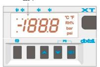
SET: To display and modify target set points; in programming mode it selects a parameter or confirm an
